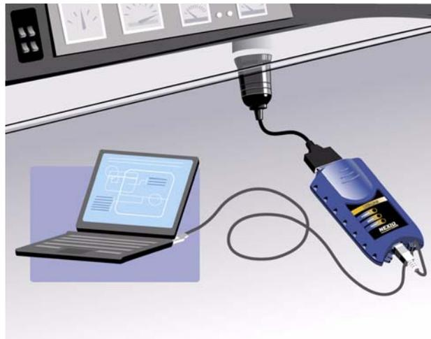
Figure 3.2 Connecting to a Notebook Computer Using a USB Cable
